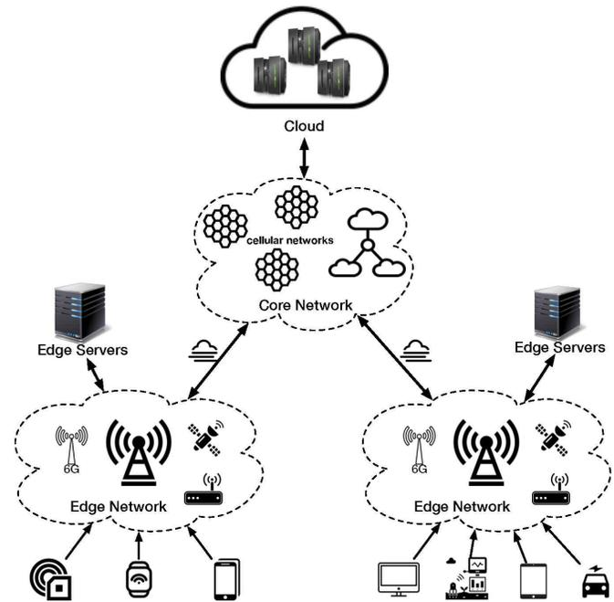
Fig. 2. Architecture of Edge Computing
