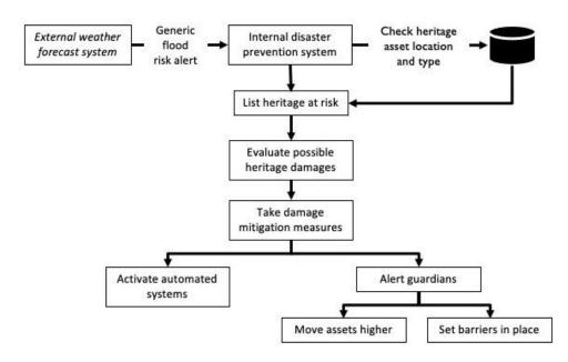
Figure 3. Schema of direct action activated by an automatic alert system based on HDT data.
