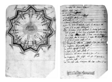
**Figure 8.** Planning the Nicosia fortress by Giulio Savorgnan: measurements of the fortress and detailed description and measurements of each enceinte component [32].
