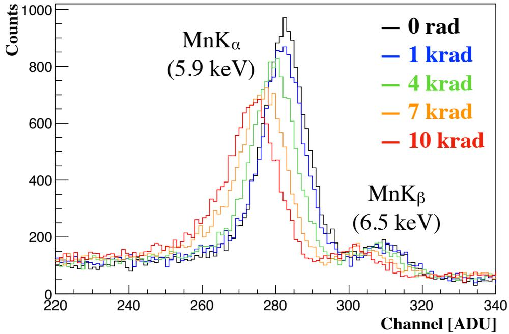
**Fig 3**  $^{55}\text{Fe}$  energy spectra of XRPIX6C before and after X-ray irradiation. The horizontal axis is uncorrected pulse height in Analog-to-Digital Unit (ADU) and the vertical axis is the number of counts.
