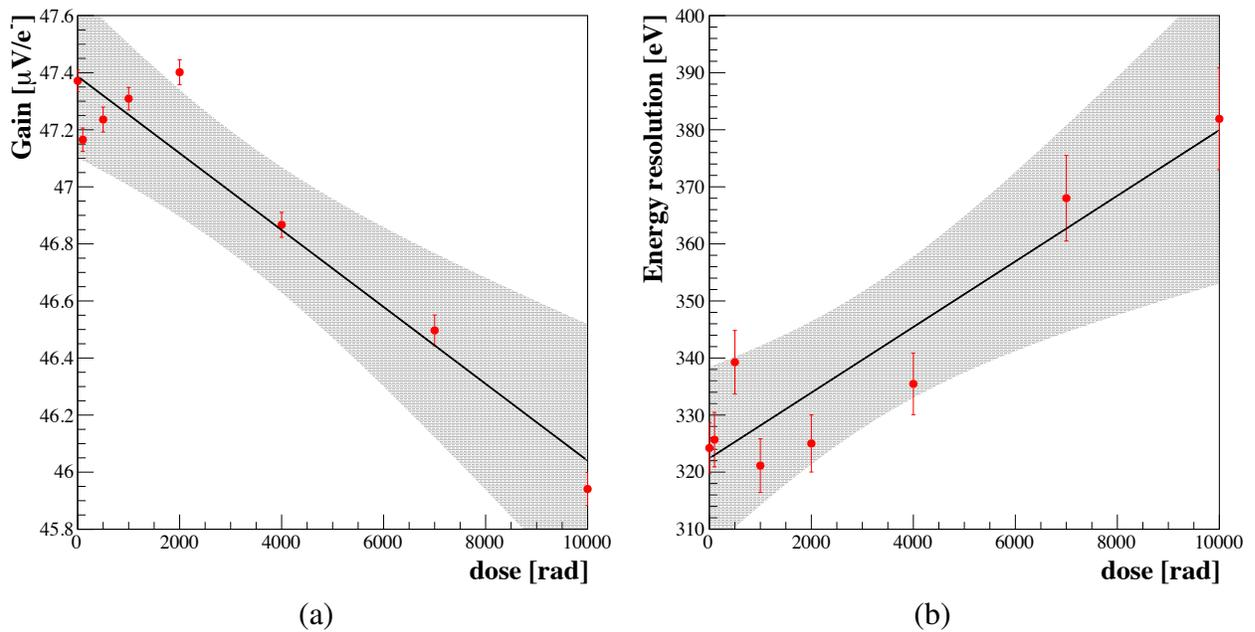
**Fig 4** (a) Conversion gain and (b) energy resolution of XRPIX6C as a function of dose level. Solid lines and shaded regions indicate the best fit linear functions and 95% confidence intervals, respectively. The confidence intervals are calculated on the assumption of Gaussian uncertainty of the data.
