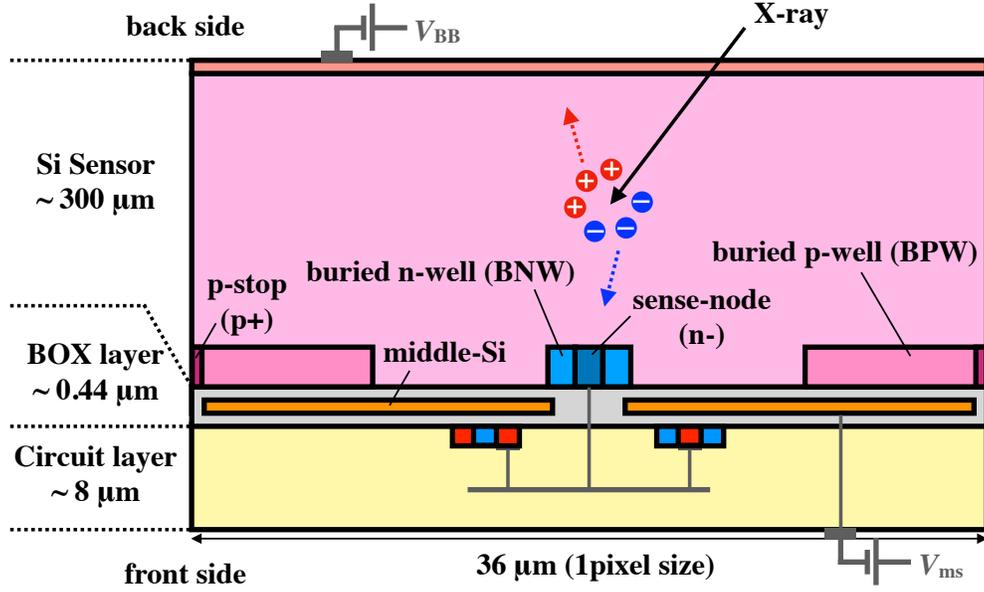
Fig 1 Schematic cross sectional view of XRPIX6C with D-SOI structure.
