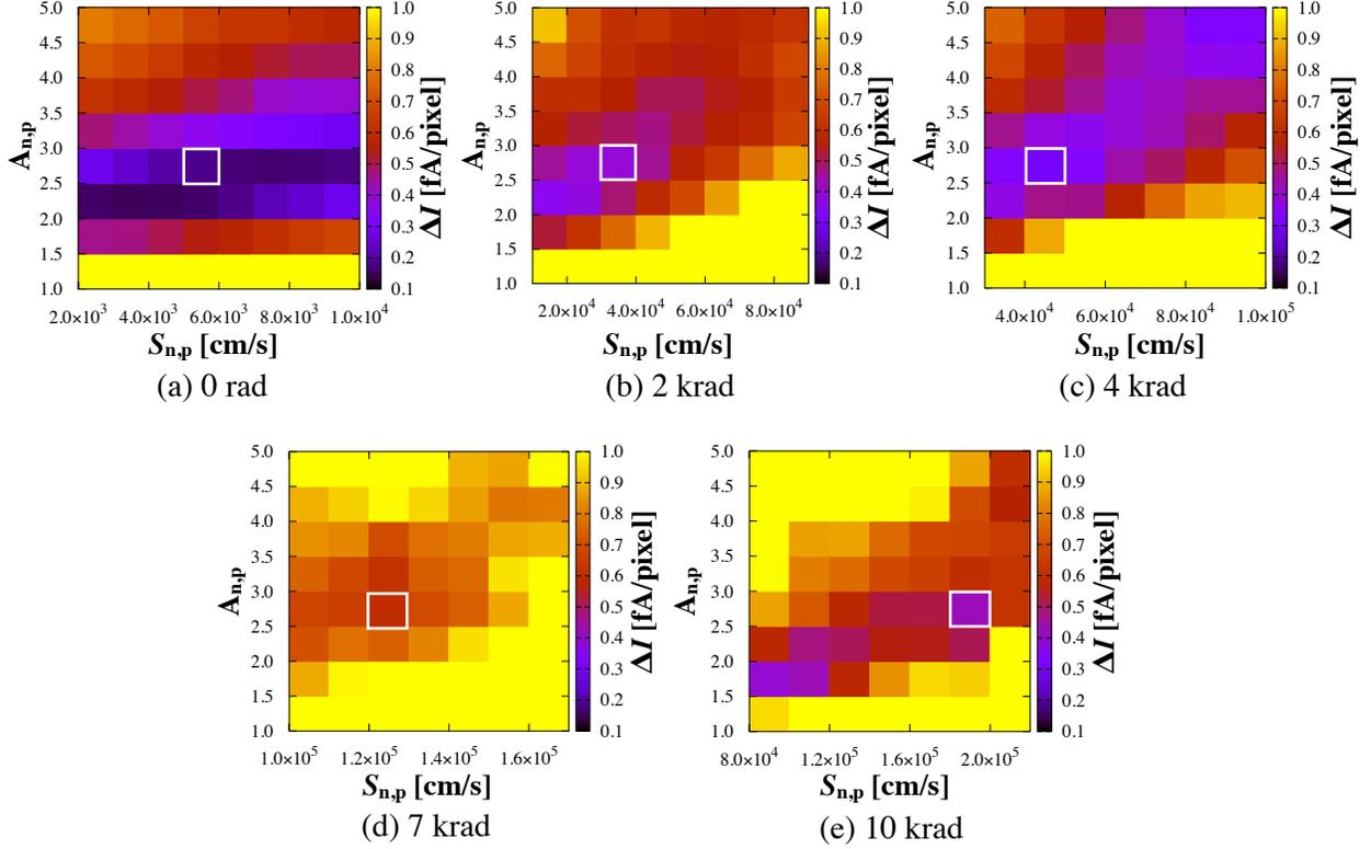
**Fig 9** The difference between the measured and simulated dark current  $\Delta I$  as a function of the simulation parameters  $S_{n,p}$  and  $A_{n,p}$ . The white squares indicate the best parameters which have a lowest  $\Delta I$  for each dose.
