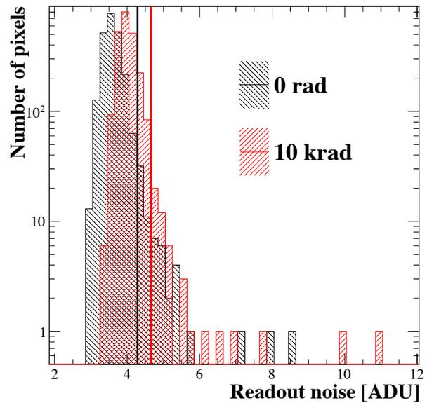
**Fig 7** Distributions of readout noise in each pixel of XRPIX6C before and after the X-ray irradiation. The noisy-pixel thresholds at  $3\text{-}\sigma$  are shown in black (0 rad) and red (10 krad) vertical thick solid lines.
