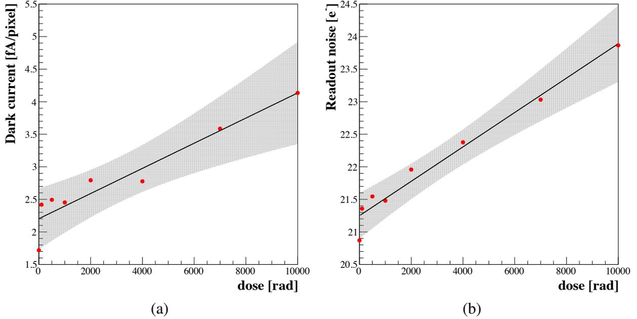
**Fig 5** (a) Dark current and (b) readout noise of XRPIX6C as a function of dose level. Best fit linear functions and 95% confidence intervals are overplotted similarly as in Fig. 4.
