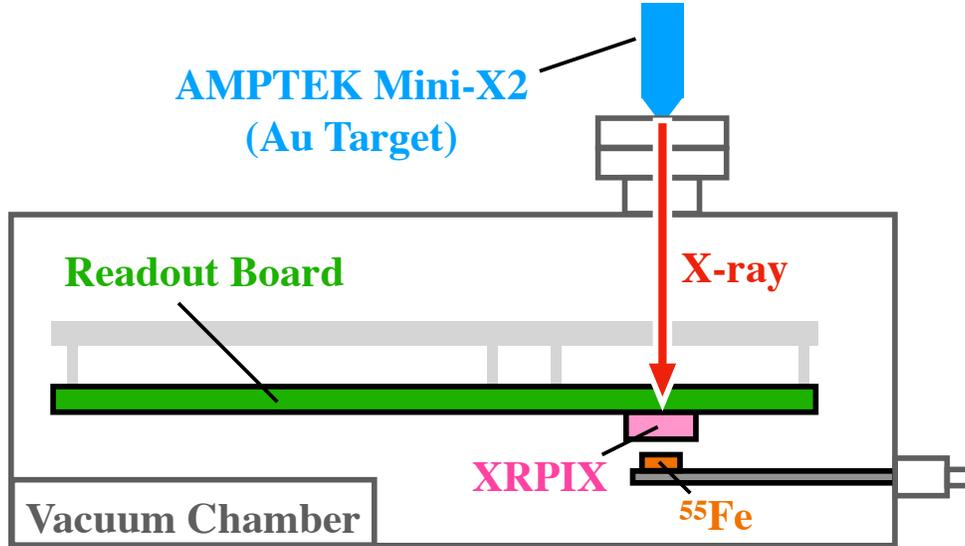
**Fig 2** Schematic view of experimental set up. We irradiated X-rays on the back side of XRPIX by using an X-ray tube, and irradiated X-rays of <sup>55</sup>Fe on the front side to evaluate the performance of XRPIX.
