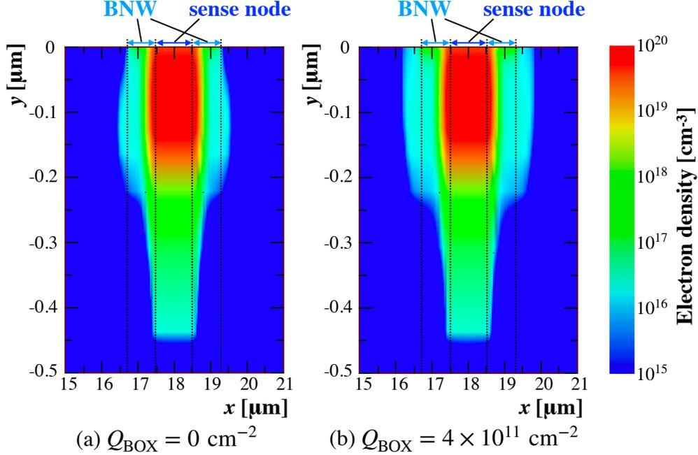
**Fig 12** The electron density distribution near the Si/SiO<sub>2</sub> interface ( $y = 0$ ). The left panel and right panel are the case with and without  $Q_{\text{BOX}}$ , respectively.
