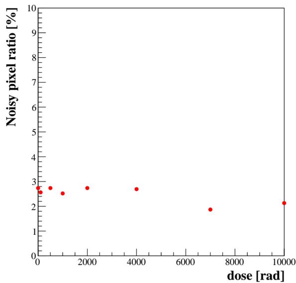
**Fig 6** Noisy pixel ratio of XRPIX6C as a function of dose level.
