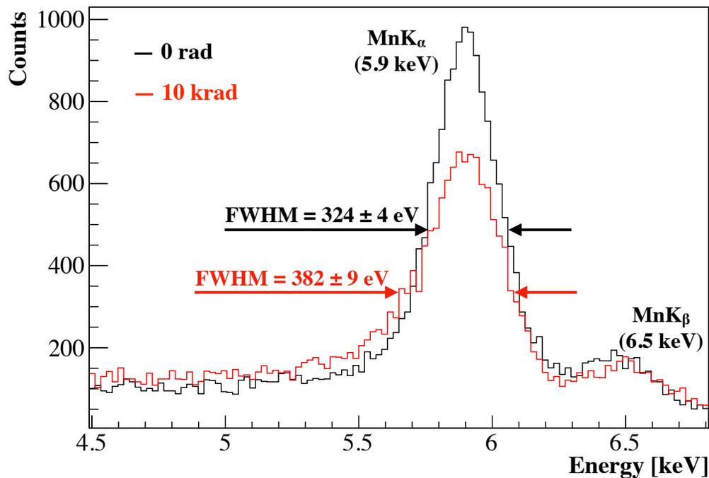
**Fig 8**  $^{55}\text{Fe}$  energy spectra of XRPIX6C corrected for the gain degradation before and after X-ray irradiation. The horizontal axis is the X-ray energy and the vertical axis is the number of counts. The tail structure increased at 10 krad compared with pre-irrad.
