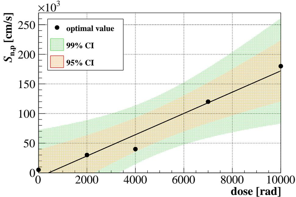
**Fig 10** The optimal values of  $S_{n,p}$  as a function of dose level. The solid line indicates the best fit linear function. The shaded regions represent its confidence intervals for 95% and 99%.
