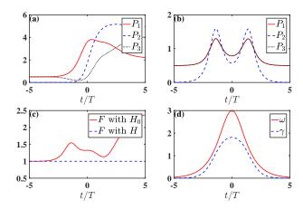
FIG. 3. (Color online) Time evolution of the Populations on  $|1\rangle$  (solid red line),  $|2\rangle$  (dashed blue line), and  $|3\rangle$  (black dotted line) driven by (a) the original Hamiltonian  $H_p(t)$  and (b) the CD driving Hamiltonian  $H_{tp}(t)$ ; (c) Time evolution of the fidelities on  $|\psi_0(0)\rangle$ ; (d) Shapes of  $\omega$  and  $\gamma$ . The parameters are chosen as  $T = 1/\Omega_0$ .
