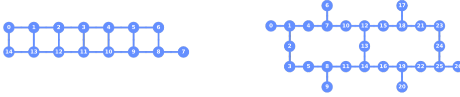
Figure 3: The square-lattice architecture of the Canary-family public-access 15-qubit ibmq_16_melbourne chip (left) and the heavy-hexagonal lattice of the Falcon-family premium-access 27-qubit ibmq_montreal chip (right) featuring lower-degree vertices.
