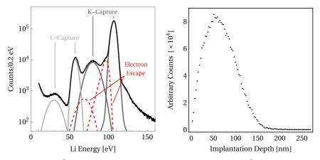
**Fig. 1** The measured <sup>7</sup>Li recoil spectrum (black) shows four peaks for the different <sup>7</sup>Be decay channels. Fits to the four decay channels and to the observed electron escape tails from the K-Capture peaks are shown (color online). Other fit features not shown. Figure adapted from [1] **Fig. 2** SRIM simulated ion depth distribution from a 25 keV ion implantation[2] at TRIUMF-ISAC
