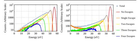
**Fig. 3** Impulse response to a 56 eV Auger electron from a fixed 10 nm implantation depth (left) and from an initial depth distribution derived from the SRIM simulation in Figure 2 (right), broadened to match the detector resolution (color online). Note the deviation from an EMG tail shape caused by 2+ electron escape, particularly at  $\sim$ 10 eV below the primary peak.
