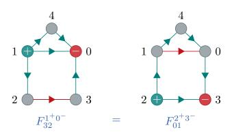
FIG. 7. Symmetry of current in a DC resistor network. Flow from vertex 2 to 3 due to a constant current source placed across (1,0) (positive at 1, negative at 0) is the same as the current from 1 to 0 due to a constant current source placed across (2,3) (positive at 2, negative at 3).
