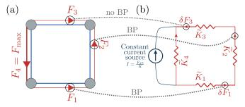
FIG. 3. Detecting all Braessian edges in a network using the resistor equivalence. The edges for which the original flow and the current flow in the resistor network are *in the same direction* are Braessian. The edges for which these two are in the opposite direction are not Braessian.
