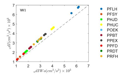
Supplementary Figure 3. Intensity of the W1 wave determined using the 2-D approximation for flow velocity (y-axis) or the full 3-D Womersley solution. Although there is a small quantitative difference in absolute values, there is a strong linear relation between the two estimates.
