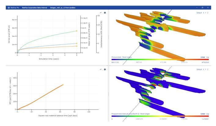
Example simulation that does not use the 'submesh fractal D' setting.
