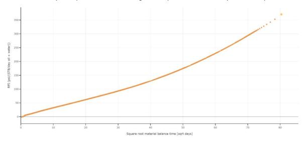
Rate-transient analysis plot from a simulation using time-dependent conductivity loss Option 2. The upward curvature is caused primarily by the conductivity loss.
