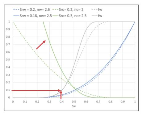
Figure 8.16 – Making relative permeability adjustments to make oil permeability more sensitive to saturation changes.
