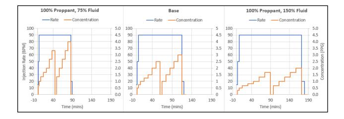
All three cases have the same volume of proppant pumped, but total fluid is changed by modifying proppant concentration.
