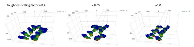
Figure 8.2 – Change in fracture dimensions with toughness scaling factor.
