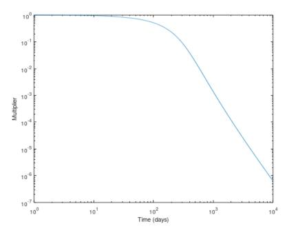
Conductivity multiplier versus time using time-dependent conductivity loss with Option 2.
