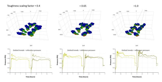
Figure 8.3 – Change in fracture dimensions and treating pressure with toughness scaling factor.
