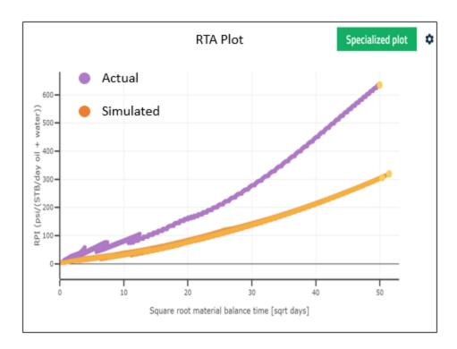
We can see that the actual data exhibits a steeper initial slope and bends upward more aggressively than the simulated data. The slope of an RTA trend is inversely proportional to the product of fracture area and the square root of permeability. Figure 8.13 shows how assuming the fracture area is matched between the actual and simulated data, we can calculate the permeability change required in our model.
