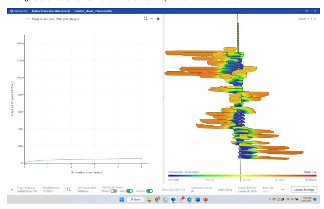
The results indicate that cross-flow during stimulation is significant at 300,000 md-ft, and relatively limited at 30,000 md-ft, and very limited at 3,000 md-ft. During production, flow rates are lower than during stimulation, and so while 3,000 md-ft is enough to prevent cross-flow during stimulation, it does not prevent significant cross-flow during production. On the other hand, going down to 30 md-ft restricts flow sufficiently that cross-flow during production is also significantly reduced.
