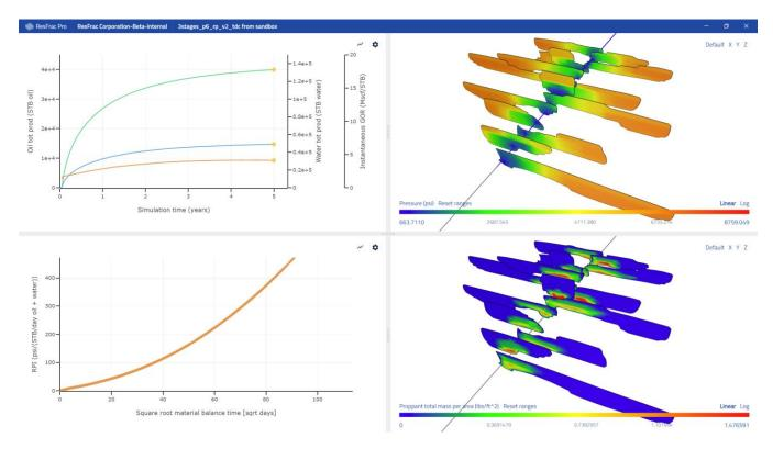
Example simulation with 'submesh fractal D' set to 0.6, and also, time-dependent conductivity loss (type 2) with a time constant of .0004 days^-1.
