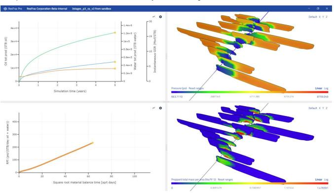
Example simulation with 'submesh fractal D' set to 0.3.
