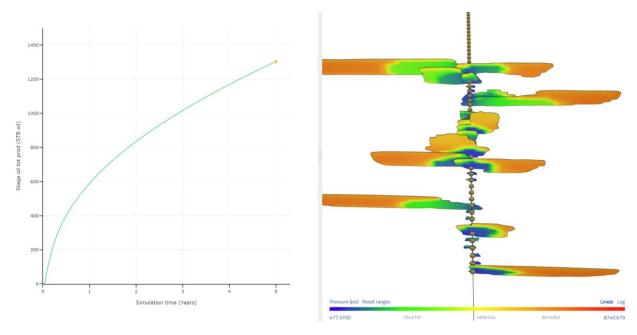
This figure shows the results with the 'transmissibility barrier' set to 3e5 md-ft.
