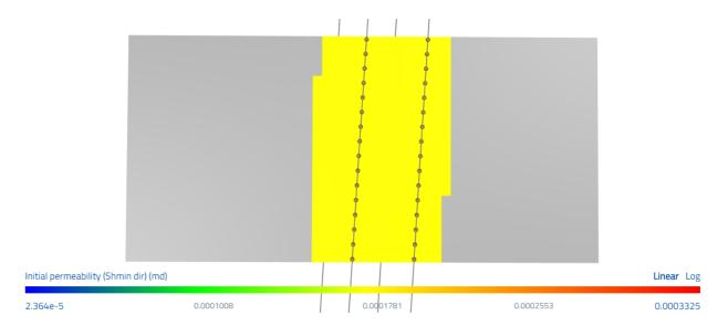
These zero perm boundaries prohibit the edge wells from draining reservoir regions that would otherwise be drained by an adjacent well. In other words, using the zero permeability cube setup above approximates the production characteristics as if that same well spacing pattern continued across the entire acreage (i.e. 10s or 100s of wells, versus four as modeled). If you do not use a 'zero perm cube,' the outer wells are likely to outperform the inner wells.
