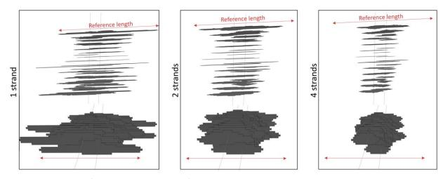
Figure 8.1 – Change in fracture dimensions with fracture strands per swarm.
