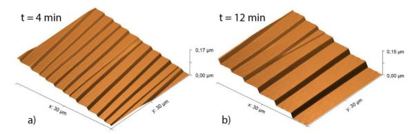
Fig.1. AFM images of the sublimating Si(111) vicinal surface, misoriented in the [11-2] direction by 0.3°, heated by step-down direct current for 4 min (a) and 12 min (b).
