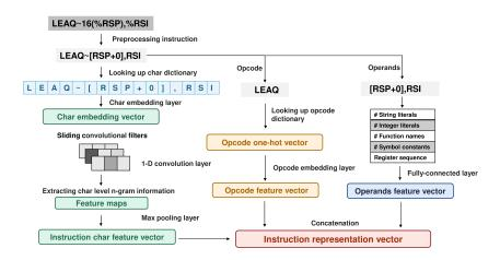
Fig. 4. Multi-feature fusion-based instruction representation process.
