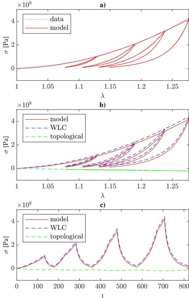
Figure 4: Comparison of the experimental and theoretical stress-strain diagrams. Our experimental data, model parameters as in Table 1. a) Overall performance of the current model. b) Separate contributions of WLC and topological stresses. c) Same as b) plotted as a function of the time order parameter  $t$  highlighting that the topological stress gives maximum relative contribution toward low stresses.
