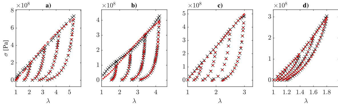
Figure 6: Comparison between modified theory and literature experiments. The evolution law includes the parameter  $\beta_{u1}$  defined in Eq.(26). Uniaxial cyclic tests on four absorbable suture threads carried out by [8]. Data are shown in black, theory including Eq.(26) is shown in red. Materials: a) Monoplus; b) Monosyn; c) Polydioxanone 2.0; d) Polydioxanone 4.0.
