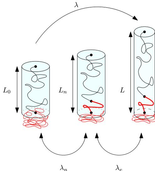
Figure 1: Cartoon of the chain deformation  $\lambda$  decomposition into an elastic and a natural stretch  $\lambda_e$  and  $\lambda_n$ , respectively. The light blue tube represents the topological constraint arising from the chain interaction within the network. The amorphous region length (thin red line outside the tube) does not contribute to the filament length  $L$  since it is expected to be small compared to the unfolded region (hidden length).
