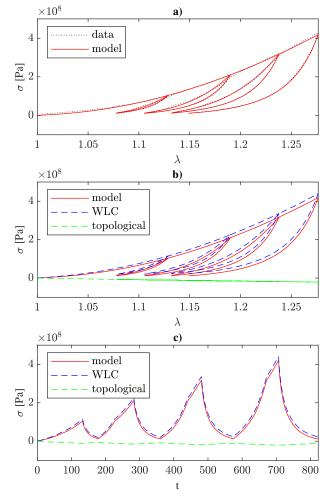
Figure 4: Comparison of the experimental and theoretical stress-strain diagrams. Our experimental data, model parameters as in Table 1. a) Overall performance of the current model. b) Separate contributions of WLC and topological stresses. c) Same as b) plotted as a function of the time order parameter t highlighting that the topological stress gives maximum relative contribution toward low stresses.
