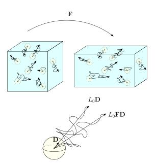
Figure 3: Micro-macro scale transition. The representative volume (light blue) contains a distribution of filaments which are isotropically oriented in space along the unit vector  $\mathbf{D}$  whose directional cosines are measured on the microsphere (yellow). The macroscopic deformation gradient  $\mathbf{F}$  stretches and rotates the filaments according to the affinity hypothesis.
