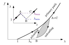
Figure 2: Filament loading history. Inset) Stretch vs time. The magenta line shows the primary path, the path AB unloading, the path BC reloading (see Eq.(8)). Main) Force vs stretch. An internal hysteresis cycle (gray) is produced along the path ABC. The residual stretch  $\bar{\lambda}_n$  is the stretch at zero force and evolves with the primary path.
