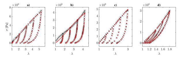
Figure 6: Comparison between modified theory and literature experiments. The evolution law includes the parameter  $\beta_{u1}$  defined in Eq.(26). Uniaxial cyclic tests on four absorbable suture threads carried out by [8]. Data are shown in black, theory including Eq.(26) is shown in red. Materials: a) Monoplus; b) Monosyn; c) Polydioxanone 2.0; d) Polydioxanone 4.0.
