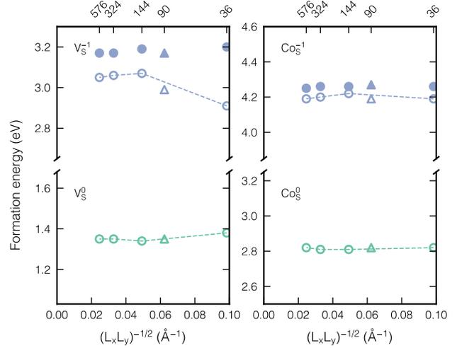
FIG. S1. Uncorrected and corrected formation energies for the  $V_S$  and  $Co_S$  defects calculated with DFT-PBE. For the series of supercells with 36, 144, 324, and 576 atoms (denoted by circles) the supercell length  $L_z = 1.6(L_x L_y)^{1/2}$ . For the 90-atom supercell (denoted by triangles)  $L_z = 1.5(L_x L_y)^{1/2}$ . For the charged defects, the uncorrected (corrected) formation energies are shown by the empty (filled) circles.
