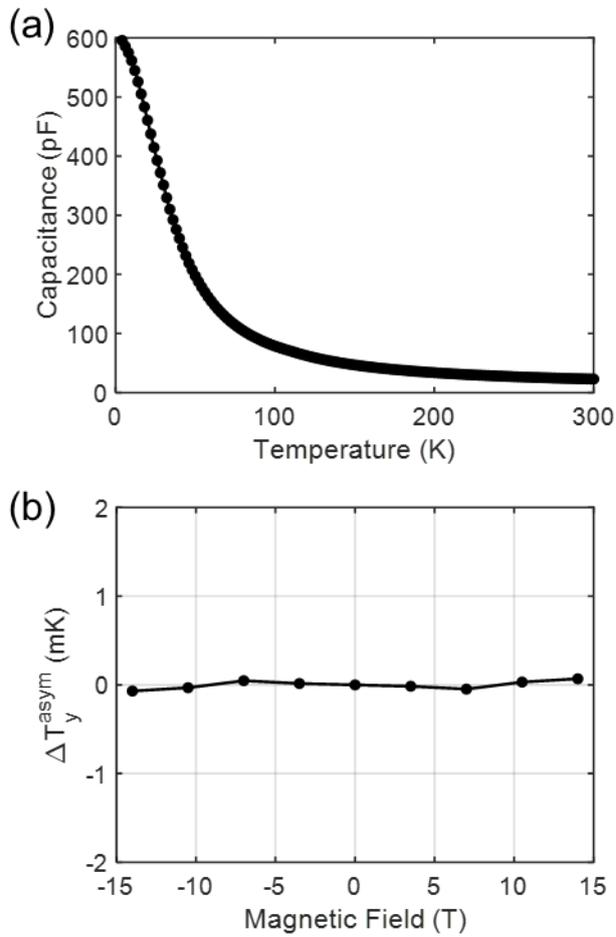
Figure 5 **Typical capacitance value of homemade SrTiO<sub>3</sub> capacitive thermometer and result of control experiment.** (a) Capacitance of SrTiO<sub>3</sub> thermometer is given as a function of temperature down to 4 K: the capacitance grows monotonically as the temperature gets lowered. (b) Antisymmetrized transverse temperature difference ( $\Delta T_y^{asym}$ ) obtained from control experiment at 20 K, in which we turned off the heat current along the sample.
