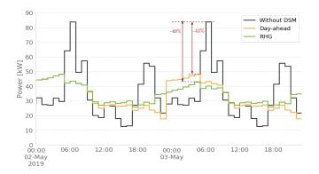
Fig. 2. Aggregate Load comparison for New York over 2 days for a set of 10 active prosumers and 5 passive consumers. Price rates  $\rho_1$ ,  $\rho_2$  are doubled from 6:00 to 10:00 and 18:00 to 22:00 to incentivize peak shaving.
