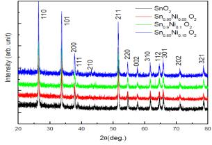
Figure 1: X-ray diffraction patterns of  $Sn_{1-x}Ni_xO_2$  (x = 0, 0.05,0.1 0.15) compound.
