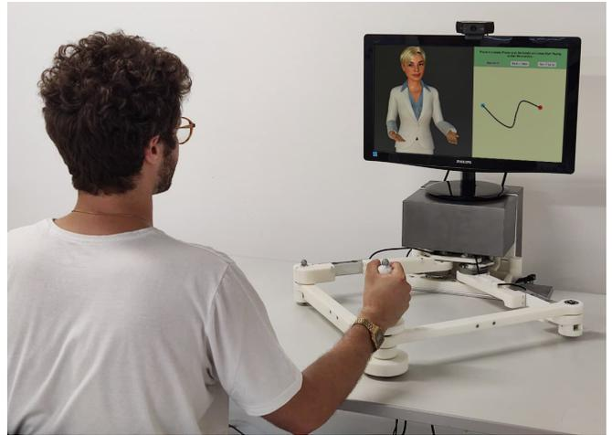
Fig. 1. Empathetic Neurorehabilitation robotic training system concept.
