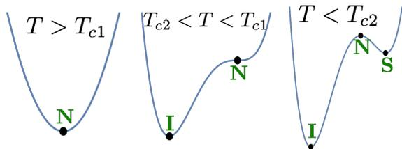
FIG. 1. Free energy profile of the electron-phonon system after the Migdal-Eliashberg theory breaks down,  $\lambda > \lambda_c$ . New order emerges [insulator (I) in this case] below  $T_{c1}$  out of the normal (N) state. Superconducting (S) stationary point appears at a lower temperature  $T_{c2}$ . At temperatures just below  $T_{c2}$ , this stationary point must be higher in energy than the insulator by continuity.
