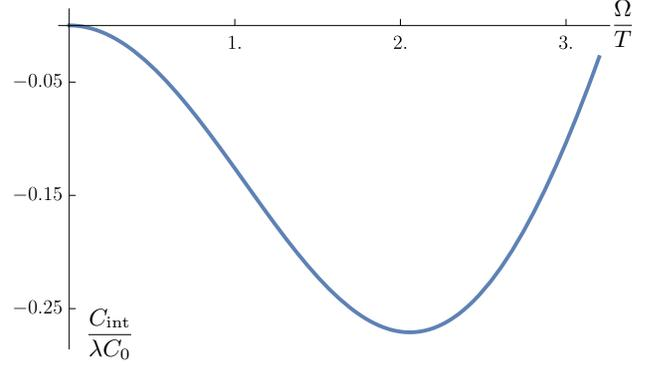
FIG. 4. Interaction contribution to the quasiparticle specific heat,  $C_{\text{int}}$  predicted by the Migdal-Eliashberg theory in units of  $\lambda C_0$ , where  $C_0$  is the specific heat of free fermions,  $\lambda$  is the electron-phonon coupling, and  $\Omega$  is the natural frequency of the Einstein phonons. Note that  $C_{\text{int}} < 0$  at any  $\lambda$  for all temperatures  $T > \Omega/3$ .
