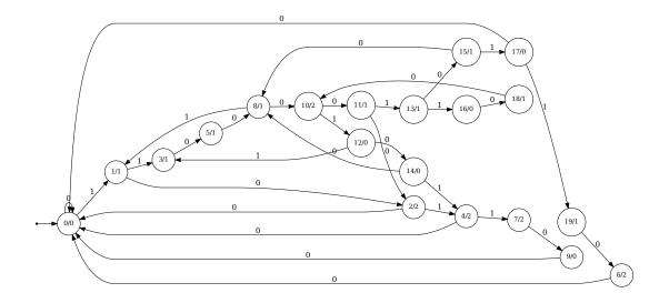
Figure 3: DFAO computing **p** in the numeration system.
