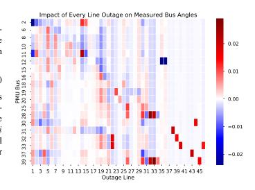
Fig. 1. An example of the  $19 \times 46$  signature map constructed using a random placement of 19 PMUs in the New England 39-bus system with 46 transmission lines. Each column corresponds to a single line outage and its incremental impact on PMU-equipped bus voltage phase angles.
