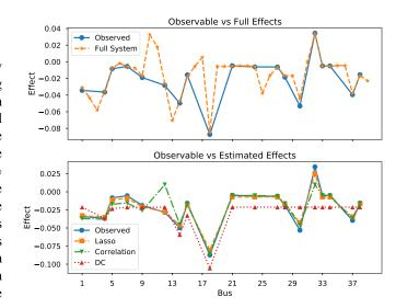
Fig. 4. Full, observed, and estimated outage impact on bus voltage phase angles after a double-line outage at line 17 and 25. 19 out of 39 buses are equipped with PMUs. The top figure shows observed noisy data with true and complete system states. The bottom figure compares the estimated phase angles changes from three methods against the observed states.
