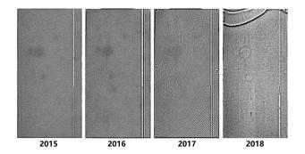
**Figure 9.** Comparison of the super-flats in four years (2015 - 2018) for the 16<sup>th</sup> CCD of the z-band.
