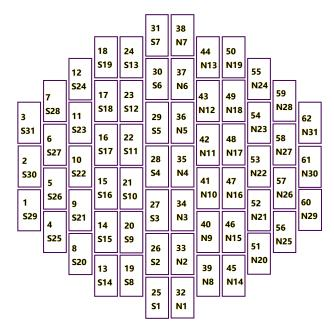
Figure 1. The distribution of the 62 CCD chips on the focal plane. Inside each chip, we show the CCD number on the upper side, and the detector position ID on the lower side.
