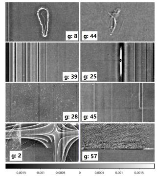
Figure 6. Each panel shows the map of the super-flat on a certain part of a CCD, the number of which is given in the corners with the band name.
