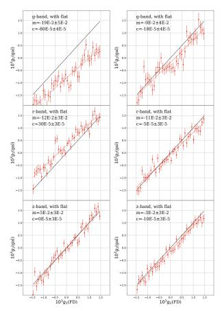
Figure 14. The results of the FD test for galaxy images in the g, r, and z band respectively. In each plot, the black solid line is the "y=x" reference, and the red dashed line is the best fit of the data points. The multiplicative and additive biases are shown in the upper left corner of each plot. The super-flat fields are used in the pipeline.
