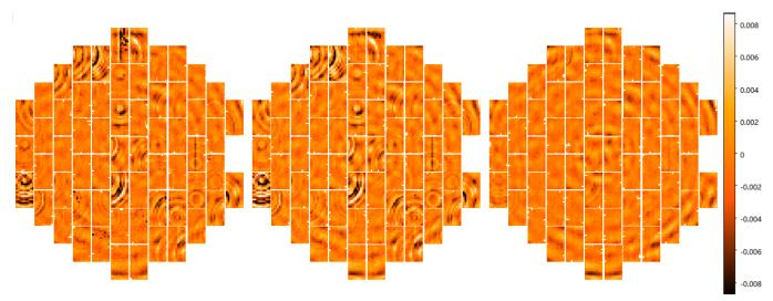
Figure 5. The residual of the PSF area from polynomial fitting up to the third order. From left to the right are the results for the g, r, and z band respectively.
