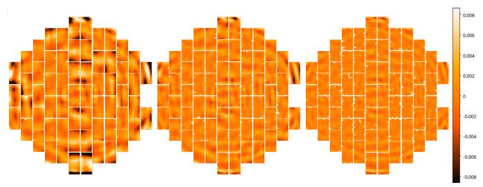
Figure 3. The residual of the  $e_1$  component of the PSF ellipticity from polynomial fitting up to the first (left plot), second (middle plot), and third order (right). The data is from the z band.
