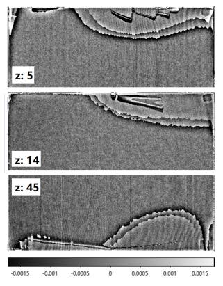
Figure 10. Defects revealed by the super-flats of year 2018 on the  $5^{th}$ ,  $14^{th}$  and  $45^{th}$  CCD in z-band.
