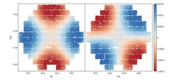
Figure 13. The distribution of the field distortion signal on the CCDs. The left and right plots show the patterns of  $g_1^f$  and  $g_2^f$  respectively. The components of  $g^f$  are defined in the coordinates of RA and Dec.
