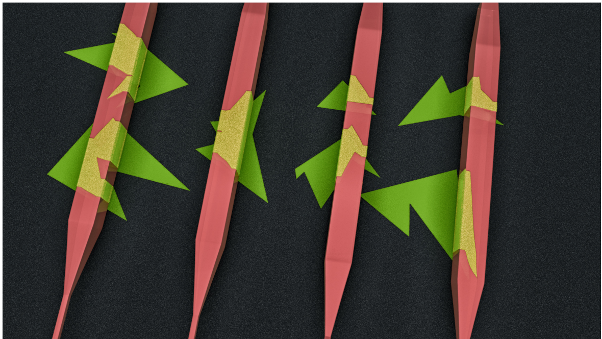
Fig. 1: Concept schematic of the MoS 2 crystal (green) grown over a Si waveguide structure (pink) via the CVD process.
