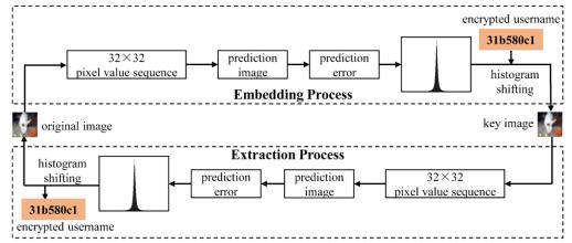
Fig. 10. Embedding and extraction process for reversible watermarking technology based on prediction error expansion
