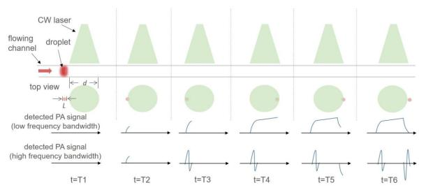
FIG. 2. The principle of passive PA effect induced by a flowing droplet (Case 2).
