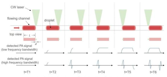
FIG. 1. The principle of passive PA effect induced by a flowing droplet (Case 1).
