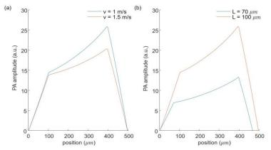
FIG. 6. The passive PA signal results under Case 2 with various key parameters. (a). PA signal with different droplet's flowing speed. (b). PA signal with different droplet lengths.
