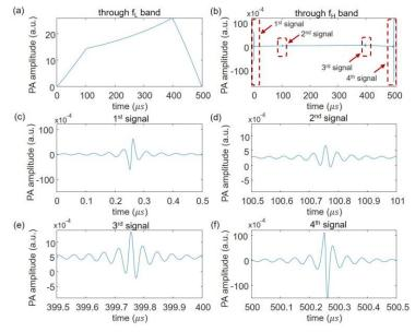
FIG. 4. The passive PA simulation results under Case 2. (a) PA signal's low-frequency component and (b) high-frequency component. (c)-(f). Zoom-in waveforms of the four PA signals in (b).
