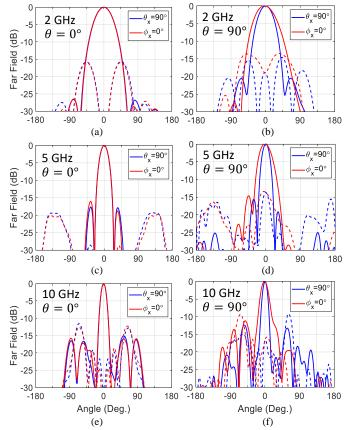
Fig. 15. Measured patterns in the  $\theta_x = 0^\circ$  and  $\phi_x = 0^\circ$  scan planes when the main beam points toward the z-axis (a), (c), (e), and x-axis (b), (d), (f). Solid lines are co-pol and dashed lines are cross pol.
