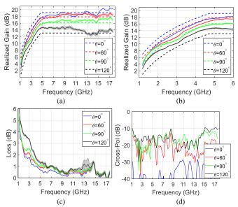
Fig. 11. Measured performance. (a) Realized gain when the beam points toward different elevation angles. (b) Zoomed in view of the gain from 1-6 GHz. (c) Combination of mismatch and radiation efficiency loss. (d) Cross-pol in the scan direction. In all cases, the array is scanned to every azimuth angle. In (a)-(c), the linewidth correspond to  $\pm 1$  standard deviation across azimuth.
