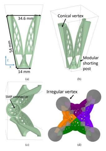
Fig. 2. (a)-(c) Different views of the hemispherical single-pol Vivaldi element. (d) Example illustrating how Vivaldi elements are modified to conform to the doubly curved surface.
