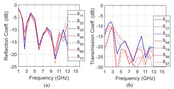
Fig. 6. Reflection coefficient (a) and transmission coefficient (b) of the antenna ports labelled in Fig. 5.
