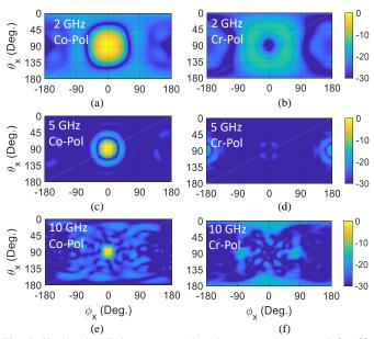
Fig. 7. Simulated radiation patterns when the array points toward  $\theta = 0^{\circ}$ . Patterns are plotted on a modified coordinate system  $\theta_x$  and  $\phi_x$ , which has the *x*-axis pointing in the same direction as the main beam.
