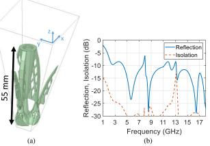
Fig. 3. (a) Dual-polarized Vivaldi unit cell. (b) Simulated active reflection coefficient and orthogonal port isolation.
