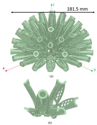
Fig. 4. (a) Designed Hemispherical Vivaldi array. (b) One of the 20 modules comprising the array.
