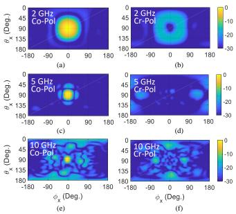
Fig. 14. Measured radiation patterns when the array points toward  $\theta = 0^{\circ}$ . Patterns are plotted on a modified corrdinate system  $\theta_x$  and  $\phi_x$ .
