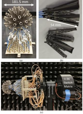
Fig. 10. (a) Fabricated array. (b) Two of the 20 modules comprising the array. (c) Array mounted on the spherical far field antenna measurement system.
