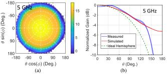
Fig. 12. Measured realized gain vs scan angle at 5 GHz. (a) Gain vs. scan angle in the u, v coordinate system. (b) Average gain vs. elevation angle. The linewidth corresponds to the standard deviation across azimuth.
