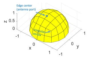
Fig. 1. Quadrilateral mesh that serves as the basis for the antenna element placement on a hemispherical array
