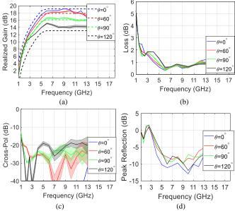
Fig. 9. Simulated performance. (a) Realized gain when the beam points toward different elevation angles. (b) Combination of mismatch and radiation efficiency loss. (c) Cross-pol in the scan direction. (d) Peak active reflection coefficient. In all cases, the array is scanned to every azimuth angle. In (a)-(c), the linewidth corresponds to  $\pm 1$  standard deviation across azimuth.
