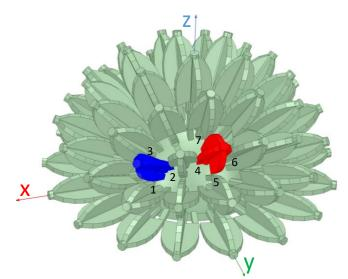
Fig. 5. Simplified array model that is simulated to estimate antenna performance. The scattering parameters of the ports connected to the blue and red vertices are plotted in Fig. 6.
