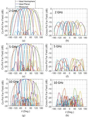
Fig. 16. Measured gain when the array is scanned to different elevation angles in the  $\phi = 0^{\circ}$  plane. The patterns are normalized by the peak gain of the  $\theta = 0^{\circ}$  case.
