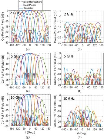
Fig. 8. Simulated gain when the array is scanned to different elevation angles in the  $\phi = 0^{\circ}$  plane. The patterns are normalized by the peak gain of the  $\theta = 0^{\circ}$  case.
