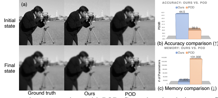
Figure 5: Image processing: comparison with POD. Ground truth solution uses P = 65,536 pixels. (a) Visually, our approach better captures the sharp initial state and the smoothed final state than POD. (b) Quantitatively, CROM obtains a higher PSNR than POD ( \uparrow the higher the better). (c) Our approach also uses an order-of-magnitude less memory than POD ( \downarrow the lower the better). Both POD and our approach use the same latent space dimension ( r = 3 ).
