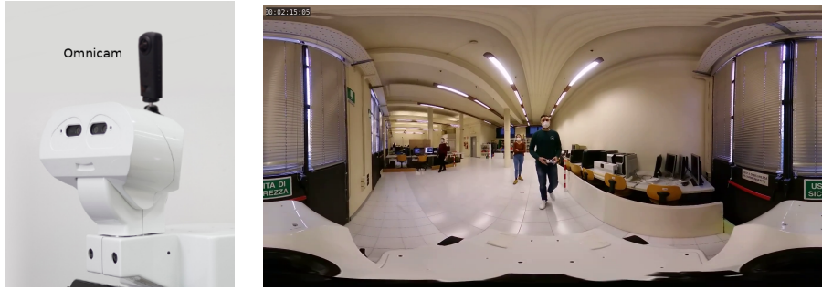
Fig. 1: (Left): The dual-fisheye omnidirectional camera mounted on the robot used in the experiments; (Right): an example of equirectangular panoramic image acquired during the experiments. This image is obtained by applying a cylindrical projection to the two images acquired by the fisheye cameras and by a subsequent image stitching phase.
