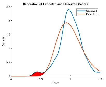
**Figure 3:** The observed curve shows the distribution of nearest neighbor feature scores generated in the previous stage. The expected curve is generated by fitting a lognormal curve to the distribution. The red region indicates students with exceedingly low independence of effort based on their deviation from the expected distribution.
