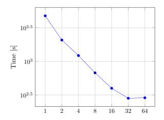
Figure 10: Execution time (in seconds) with up to 64 MPI processes for the invinterp problem, solved with thick-restart Lanczos and hypre-preconditioned LSQR.
