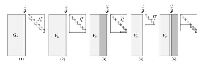
Figure 2: Illustration of the five steps of thick restart in SVD: (1) initial Lanczos factorization of order k, (2) solve projected problem, (3) sort and check convergence, (4) truncate to factorization of order r, and (5) extend to a factorization of order k.
