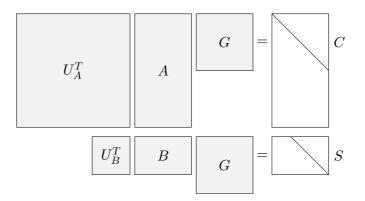
Figure 1: Scheme of the GSVD of two matrices A and B, for the case m > n and p < n.
