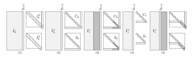
Figure 3: Illustration of the five steps of thick restart in GSVD: (1) initial Lanczos factorization of order k, (2) solve projected problem, (3) sort and check convergence, (4) truncate to factorization of order r, and (5) extend to a factorization of order k.
