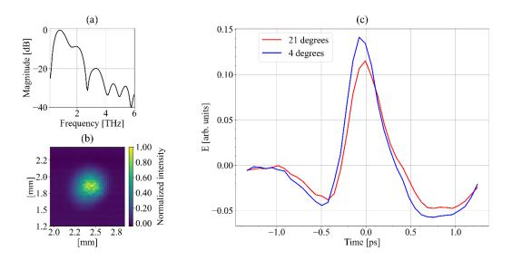
Figure 1. Terahertz transmission by liquid water in a static cell with diamond windows. a) Example spectrum of the terahertz source. This frequency-dependent spectrum is obtained by Fourier transformation of a typical terahertz field transmitted by an empty path, i.e., without the static liquid cell.
