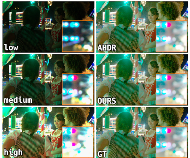
Figure 1. Qualitative comparison from our validation split comparing the AHDR Baseline with our technique. Our solution effectively merges the three input brackets and provide high quality outputs, free of noise or saturated areas. Moreover, effectively achieves higher fidelity on the zoomed areas when compared with the ground truth sample.
