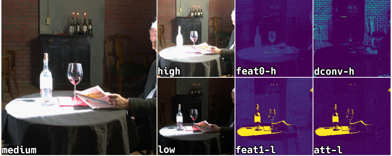
Figure 7. Qualitative representation of the behavior from the main components of our system. feat0-h is a single activation channel from Z_3^0 , and dconv-h is the same channel result after applying the Deformable Convolutional Block. dconv-h represents the effective minimization of details from the over-exposed regions of the table, while enhancing details from the background wall. At the bottom, feat1-l is a single activation channel from Z_1^0 while att-l is the same channel after applying the Spatial Attention Block. Att-l despite being at a fourth of the original resolution, is able to retain the well-exposed details from the table, while representing an accurate reduction of the over-exposed details from the background wall.
