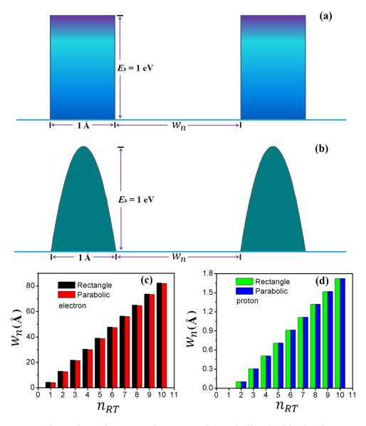
FIG. 2. Schematics of rectangular (a) and parabolic double barriers (b). The inter-barrier spacing of RT ( $w_n$ ), as a function of resonance number ( $n_{RT}$ ), for electron (c) and proton (d) across the double barriers, at incident energy E = 0.5 eV.
