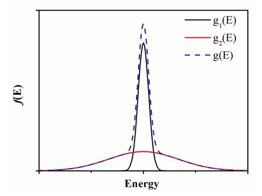
**FIG. 8.** Schematic diagram for the kinetic energy distribution (f(E)) of identical particles in microcanonical ensembles: Particle groups of high monochromaticity ( $f(E) = g_1(E)$ ), low monochromaticity ( $f(E) = g_2(E)$ ), and their superposition ( $f(E) = g(E) = g_1(E) + g_2(E)$ ).
