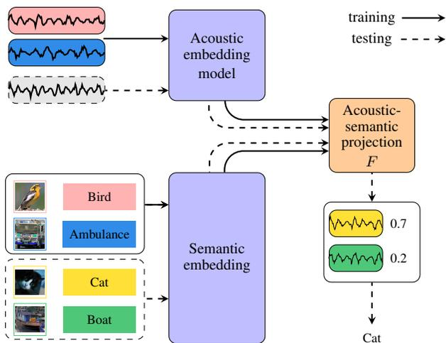
Fig. 1. Zero-shot audio classification using visual semantic information. Training is represented in solid line and testing in dashed line. Sound classes *bird* and *ambulance* are used during training and *cat* and *boat* are used in testing.
