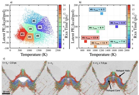
Figure 2: Molecular descriptors (a) and cluster centroids (b) colored by  $\tau_{Rxn}$  plotted in T-U<sub>latent</sub> space. (c) Spatial mapping of clustered molecules about the hotspot during and after its formation. Molecules are colored by cluster ID following the convention in panels a and b, with non-clustered molecules colored white.
