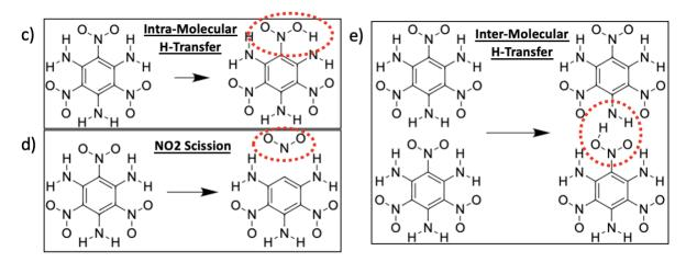
*SM- Figure 3: Schematics of the primary* 1<sup>*st*</sup> *step reaction paths for TATB.*
