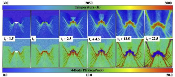
Figure 1: Time history of roto-vibrational temperature and 4-body PE in a reacting pore-collapse hot spot in TATB. The time origin  $t_o$  corresponds to complete collapse of the pore, with time offsets given in picoseconds.
