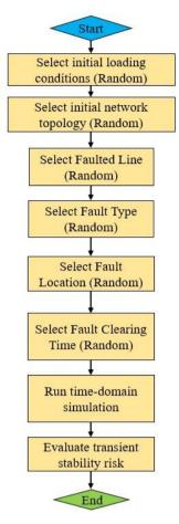
Fig. 2. Framework for probabilistic TSA
