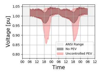
Fig. 4. When subjected to only non-PEV loads, the voltages of the feeders remained between the ANSI voltage threshold. However, PEV uncontrolled charging added significant load to the phase 2 lines, which caused the minimum voltage to drop well below 0.95 p.u. and reach a minimum of 0.85 p.u.
