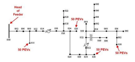
Fig. 2. IEEE 34 bus feeder, which is a canonical example of a long lightly loaded feeder. Fifty PEVs charge on nodes 810.2, 826.2, 856.2, and 838.2. Node 856.2 is used for comparing scenarios.
