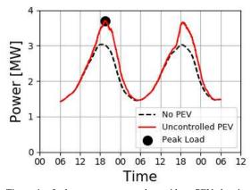
(a) Timeseries feeder power over two days without PEV charging and with uncontrolled PEV charging. The feeder peak with uncontrolled PEV load occurred at 19:29 on the first day.
