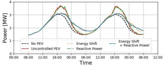
(a) The feeder profiles over a two-day period in the five simulation scenarios had similarties and differences depending on the control approach. The reactive-power control approach matched well with the uncontrolled case because very little change in active power occurred. The energy-shift and energy-shift + reactive-power approaches had a similar peak with the no-PEV case, but had larger power draws during the night.
