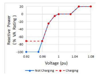
Fig. 1. Volt-var curve used in the Reactive Power Support control strategy. The sign convention views PEV as a load and not a generator, negative reactive power is capacitive load that supplies Q and positive reactive power is inductive load that consumes Q.
