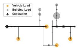
(b) PEV and non-PEV load magnitudes at uncontrolled PEV feeder peak. The magnitudes of the markers are proportional to the load.
