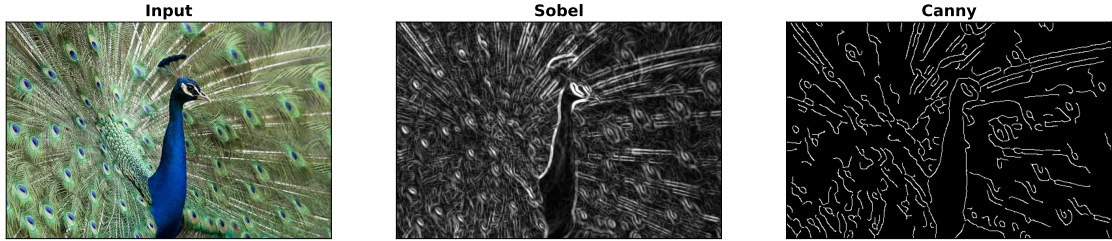
Figure 8: Comparison of different edge detection algorithms: Sobel and Canny.
