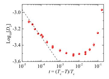
FIG. 2. Second sound diffusivity  $D_2$ , in units of cm<sup>2</sup>/s, as a function of the reduced temperature  $t = (T_c - T)/T_c$ . The experimental data (circles) are from Mehrotra and Ahlers in 1983, measured from the resonance linewidth of cw cavities [40]. The dashed line illustrates the critical behavior  $D_2 \propto t^{-\nu/2}$  near the superfluid lambda transition, with a critical exponent  $\nu \simeq 2/3$ .
