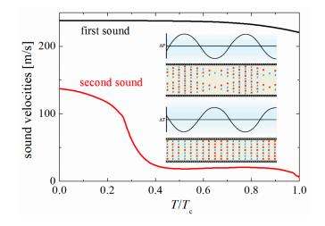
FIG. 1. First and sound velocities of superfluid helium as a function of the reduced temperature  $T/T_c$ , where  $T_c \simeq 2.17$  K is the critical temperature. The inset illustrates the characteristics of the two sounds: the in-phase motion (first sound) and the out-of-phase motion (second sound) between the normal and superfluid components, which are shown by the red circles with "n" and the blue circles with "s". Adapted from Ref. [1] and Ref. [15].
