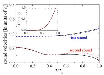
FIG. 4. First and second sound velocities of a uniform Fermi gas at unitarity (solid lines), predicted by the GPF theory. The units of the velocity is  $v_F = \hbar k_F/m$ . The uncoupled first and second sound velocities given by  $v_S$  and v are shown as dashed and dotted lines, respectively. The inset shows the Landau-Placzek ratio as a function of  $T/T_c$ . From Ref. [15].
