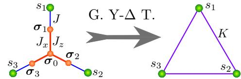
Figure 2. Schematic representation of generalized star-triangle transformation (G. Y-Δ T.) of a spin-1/2 Ising-XXZ model of decorated three-leg star onto a spin-1/2 Ising model on a triangular structure.
