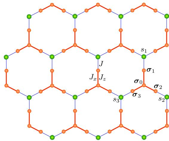
Figure 1. Spin-1/2 Ising-Heisenberg decorated honeycomb lattice, orange spheres correspond to Heisenberg spins, and green spheres denote Ising spins. Orange lines correspond to Heisenberg exchange interactions, and blue lines indicate the Ising exchange interactions.
