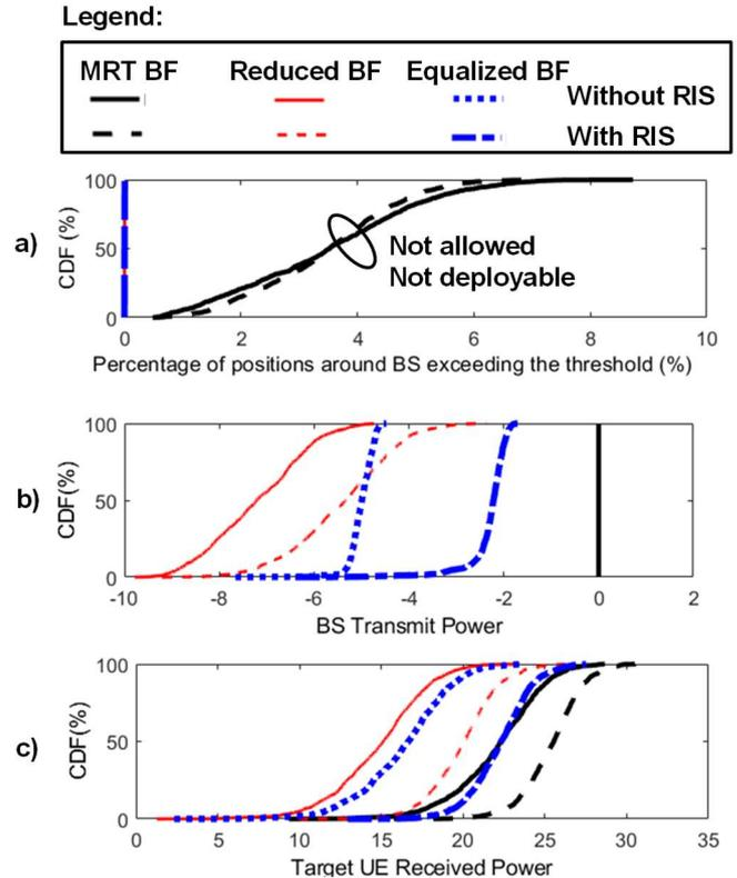
Fig. 8. CDFs of a) positions around BS (outside the limit circle and inside a  $1400\lambda$  by  $1400\lambda$  square around the BS) exceeding the threshold b) BS transmit power and c) target UE received power, assuming the same target UE is served for a long period.
