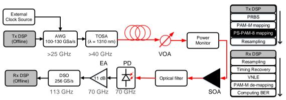
AWG: arbitrary waveform generator; TOSA: transmitter optical sub assembly; VOA: variable optical attenuator; SOA: semiconductor optical amplifier; PD: photodetector; EA: electrical amplifier; DSO: digital storage oscilloscope **Fig. 2:** Schematic of the IM/DD transmission system with transmitter and receiver-side offline DSP.
