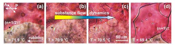
Figure 5. Phase transition on cooling from  $N^*$  (a) through unstable dynamic process ((b) and (c)) to  $N^*_F$  phase (d) in wedge-like LC cell filled with the mixture RM734:DIO (70:30) doped with 15.5 wt.% CB15.
