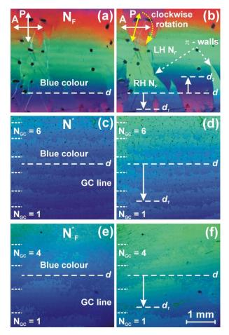
Figure 6. The shift of the interference colours in wedge-like LC cells during rotation of polarizer in the clockwise direction (GC method) for various phases: (a), (b)- basic  $N_F$  mixture at 120 °C; (c), (d) - N<sup>\*</sup> phase at 89 °C and (e), (f) - N<sup>\*</sup><sub>F</sub> phase at 84 °C of the chiral  $N_F$  mixture RM734:DIO (70:30) doped with 11.1 wt,% CB15.
