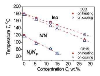
Figure 1. Phase transition temperatures between isotropic (Iso), nematic/chiral nematic  $(N/N^*)$  and ferroelectric nematic/chiral nematic  $(N_F/N^*_F)$  phases for the basic mixture 70
