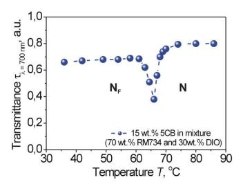
Figure 9. Optical transmittance for ferroelectric mixture  $N_F$ , based on 15 wt.% 5CB dissolved in the basic  $N_F$  mixture, consisting of two ferroelectric nematics RM734 and DIO in ratio (70:30) at 700 nm as function of temperature. The thickness of the plane-parallel LC cell was 20  $\mu$ m.
