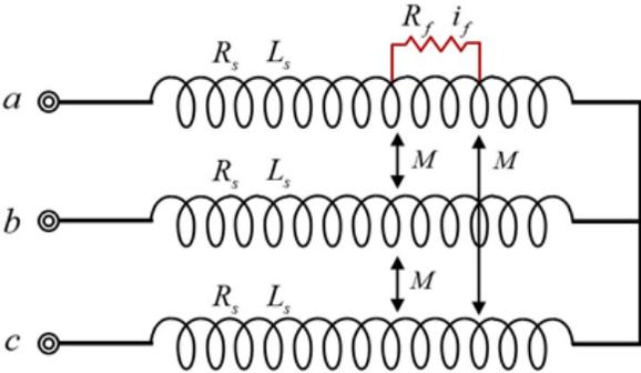
Fig. 2 Stator winding of inter-turn short circuit fault scheme
