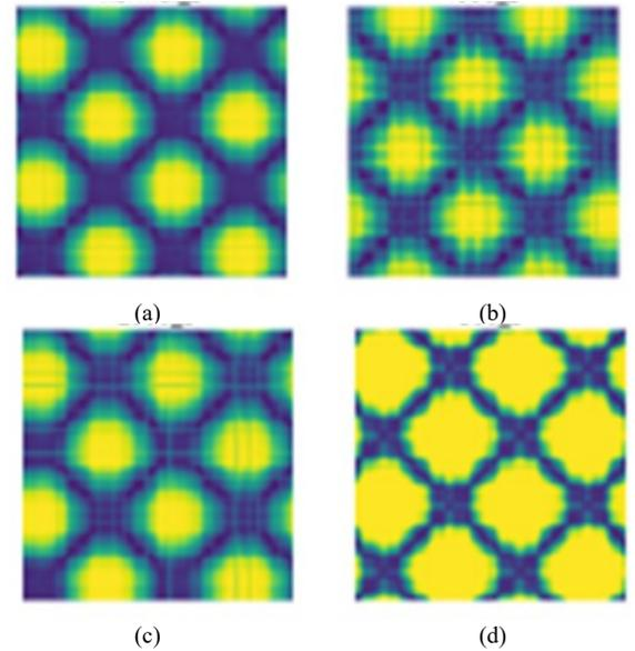
Fig. 5. RP images of stator current signals from 3.0 kW motor: (a) healthy state, (b) faulty state (1.82 %), (c) faulty state (4.33 %), and (d) faulty state (7.80 %)
