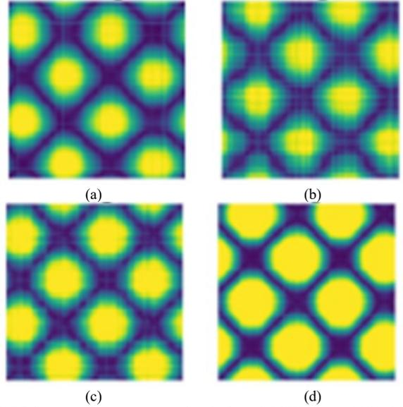
Fig. 4. RP images of stator current signals from 1.5 kW motor: (a) healthy state, (b) faulty state (1.82 %), (c) faulty state (4.33 %), and (d) faulty state (7.80 %)
