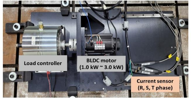
Fig. 3 Description of electric motor testbed
