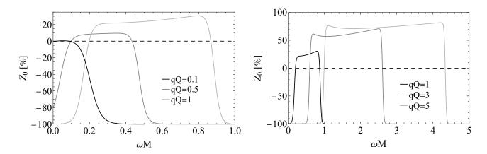
FIG. 4. Amplification factors of massless charged  $m_0 = 0$  monochromatic scalar waves for an accelerating RN BH with  $\alpha M = 0.2$ , Q = 0.99M and varying charge coupling qQ. The horizontal black dashed line designates the onset of superradiant amplification.
