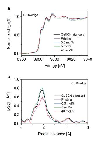
Figure S4. (a) XANES spectra at the Cu K-edge. (b) Analyzed EXAFS spectra in the R-space.
