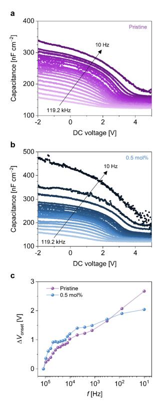
**Figure S13.** Frequency dispersion of *C-V* characteristics of metal-insulator-semiconductor (MIS) structures based on (a) pristine and (b) 0.5 mol% l<sub>2</sub>-doped CuSCN. (c) The shift in the onset voltage of the *C-V* characteristics ( $\Delta V_{onset}$ ) relative to the onset at the highest frequency (119.2 kHz).
