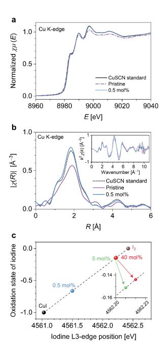
**Figure 2.** Cu K-edge (a) XANES spectra and (b) EXAFS spectra in R-space (inset, in k-space). The radial distance (R) is shown without phase shift correction. (c) Oxidation state of iodine determined from the absorption edge positions of I L3-edge XANES.
