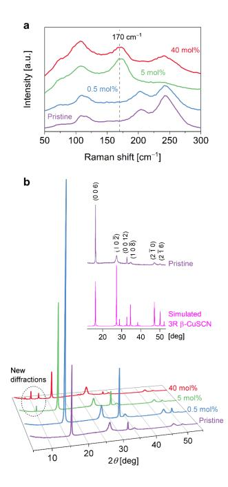
**Figure 1.** (a) Raman spectra. The peak at 170 cm<sup>-1</sup> is ascribed to I<sub>2</sub> acting as an electron acceptor. (b) X-ray diffraction data of the pristine and I<sub>2</sub>-doped CuSCN samples. (b, inset) The diffractions of the pristine sample can be matched with those from the 3R  $\beta$ -CuSCN polytype.
