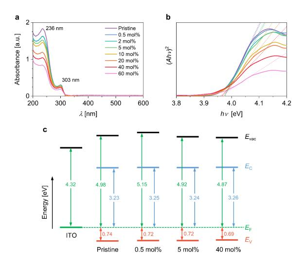
**Figure 3.** (a) Optical absorbance spectra. (b) Tauc plots for the determination of the optical band gaps. (c) Energy diagrams constructed with data from photoelectron spectroscopy (PES) and the optical band gaps.  $E_v$ : valence band edge;  $E_F$ : Fermi level;  $E_c$ : conduction band edge;  $E_{vac}$ : vacuum level.
