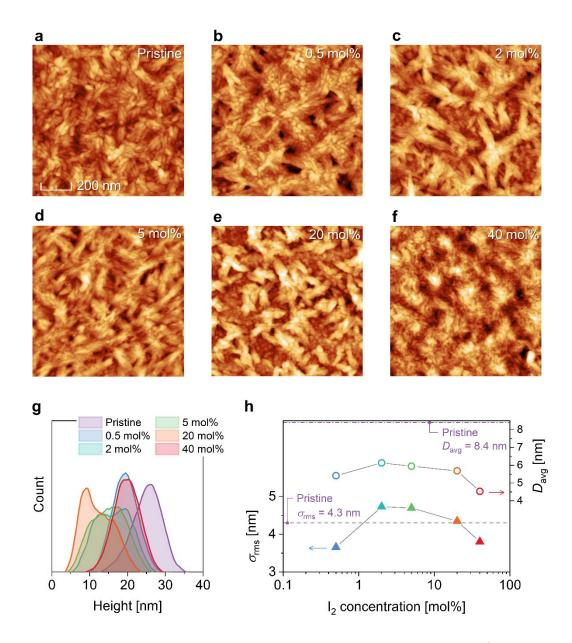
**Figure S6.** (a-f) AFM images of pristine and I<sub>2</sub>-doped CuSCN films of area of 1x1  $\mu$ m<sup>2</sup>. Analyzed data: (g) surface height histograms and (h) root-mean-squre surface roughness ( $\sigma$ <sub>rms</sub>, left y-axis, solid triangles) and average grain size ( $D_{avg}$ , right y-axis, open circles) of various I<sub>2</sub> doping conditions. The dashed lines represent data of the pristine CuSCN films:  $\sigma$ <sub>rms</sub> = 4.3 nm and  $D_{avg}$  = 8.3 nm.
