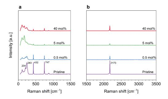
**Figure S2.** Raman spectra of pristine and  $I_2$ -doped CuSCN samples (drop-cast from DES solutions) in the (a) 0 to 1500 cm<sup>-1</sup> and (b) 1500 to 3500 cm<sup>-1</sup> wavenumber ranges.
