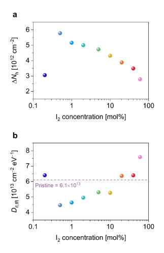
**Figure S12.** (a) The shift in the hole concentration calculated from the shift in the threshold voltage  $(\Delta N_h)$  and (b) interface trap density calculated from the subthreshold swing  $(D_{it,tft})$  of CuSCN transistors with varying I<sub>2</sub> doping concentration.
