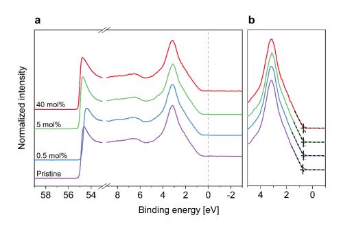
**Figure S9.** Photoemission spectra of pristine and I<sub>2</sub>-doped CuSCN films on ITO substrates measured using synchrotron radiation. (a) Full data range showing the top of the valence bands and the secondary electron cutoff edges. (b) Close-up at the top of the valence bands for the determination of the onsets.
