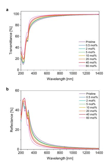
**Figure S7.** UV-Vis-NIR (a) transmittance and (b) reflectance spectra of pristine and I<sub>2</sub>-doped CuSCN thin films spin-cast on fused silica substrates.
