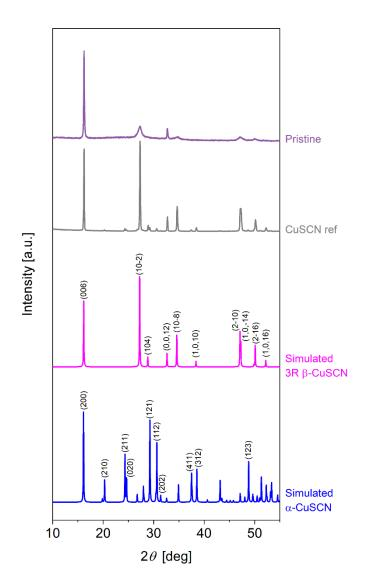
**Figure S3.** Comparison of the X-ray diffraction pattern of the prisine CuSCN sample (drop-cast from DES solution) with that of the reference CuSCN powder (99%, Sigma-Aldrich), simulated pattern of 3R  $\beta$ -CuSCN (ICSD 24372), and simulated pattern of  $\alpha$ -CuSCN (ICSD 124).
