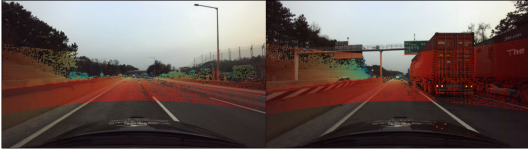
Figure 18: Examples of calibration result between the camera and Lidar, where colored points on the front images show the projected points of the corresponding LPCs.
