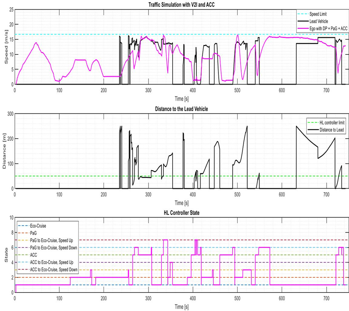
Figure 12. Traffic simulation for ego vehicle with V2I and ACC
