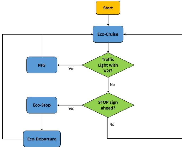
Figure 6. Flowchart for the HL controller with no traffic
