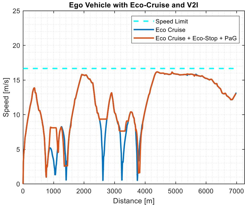
Figure 11. Ego vehicle with Eco-Cruise only and Eco-Cruise + Eco-Stop + PaG
