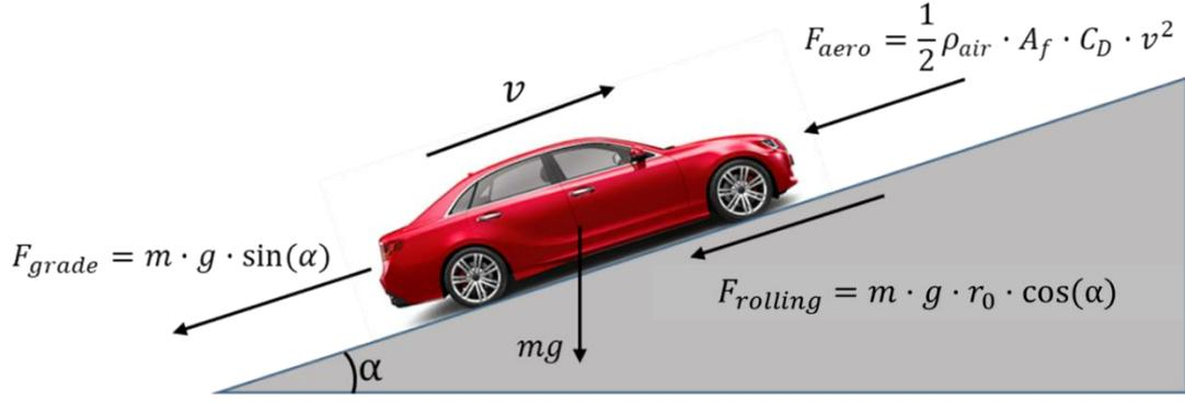
Figure 4. Road forces acting on a vehicle
