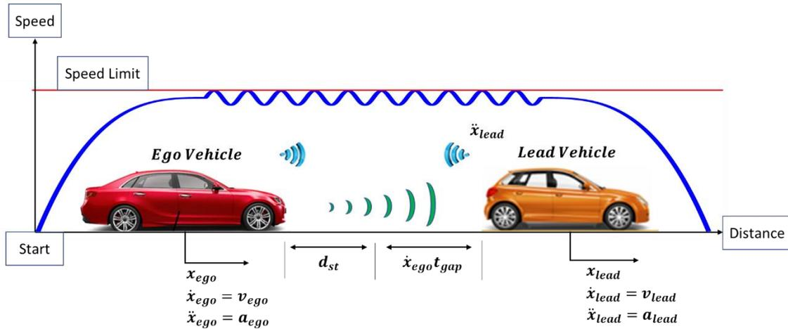
Figure 3. Car following of a CAV as an optimal control problem
