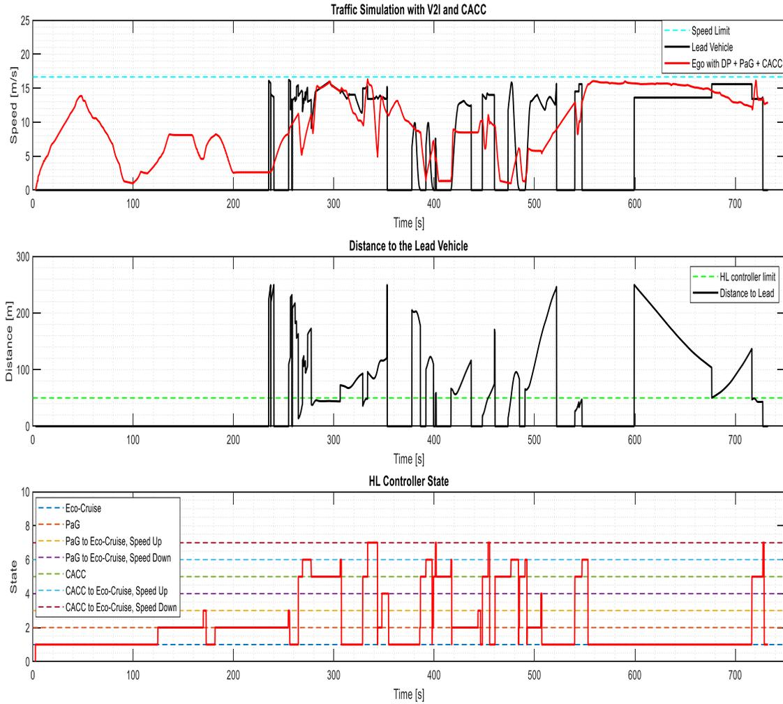
Figure 13. Traffic simulation for ego vehicle with V2I and CACC
