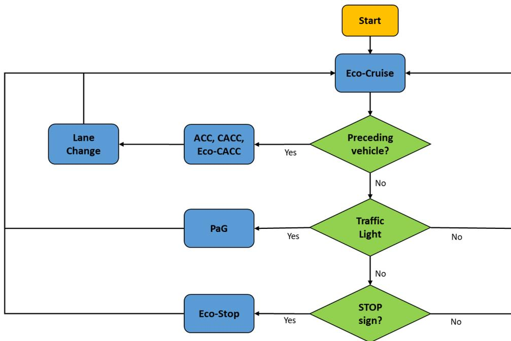
Figure 9. HL controller flowchart for traffic simulations
