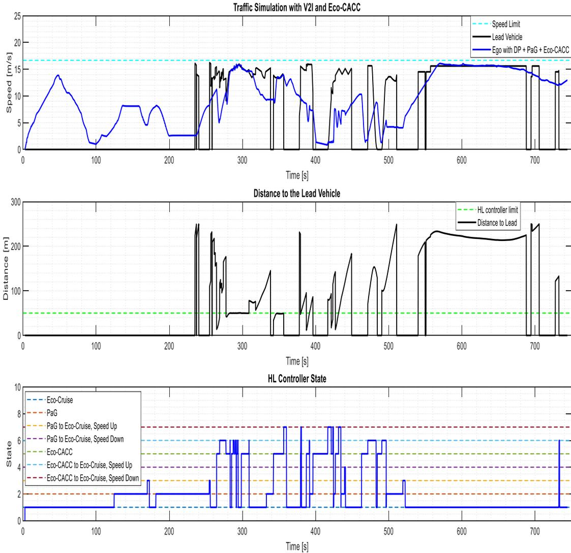
Figure 14. Traffic simulation for ego vehicle with V2I and Eco-CACC
