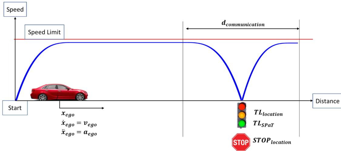
Figure 2. V2I interaction as an optimal control problem
