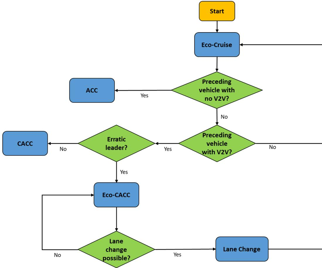
Figure 7. Flowchart for the HL controller with traffic
