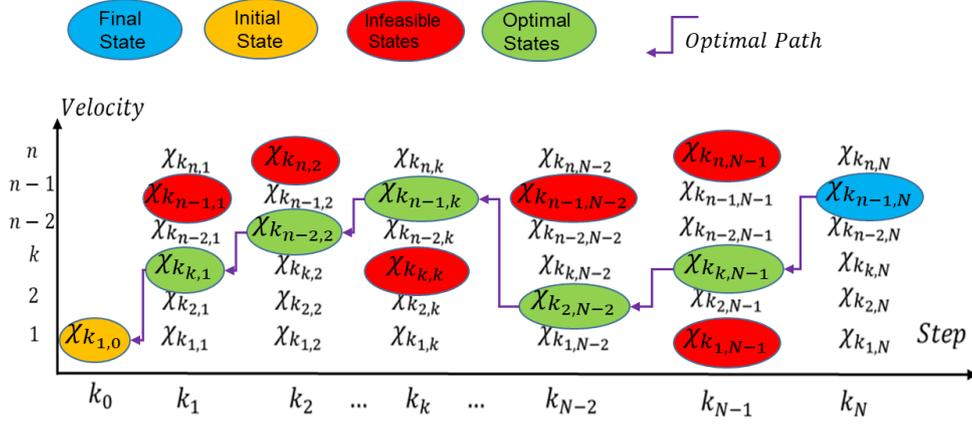
Figure 5. DP algorithm table for the optimal solution (Kavas-Torris *et al.*, 2021)
