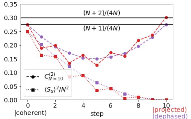
FIG. 2. Coherence parameters,  $C_N^{(2)}$  and  $\langle S_x \rangle$ , as a function of the number of qubits coupled to the ancillas, for a state with  $N = 10$  qubits and  $N_a = 3$  ancillas. The red (purple) curves refer to situation where all the ancilla are (not) postselected, leading to the creation of the state  $|\text{projected}\rangle$  ( $|\text{dephased}\rangle$ ). The horizontal lines correspond to the  $C_N^{(2)}$  values for these states, Eqs. (5)-(7).
