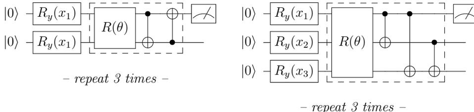
**Figure 2.** VQC circuit for the one-dimensional (left) and three-dimensional (right) datasets.
